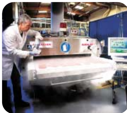
Tunnel de surgélation, Himalaya
