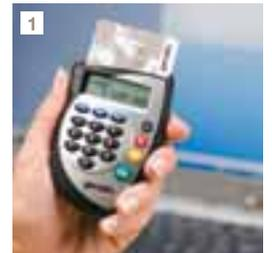
1. Our pocket-sized device provides convenient One-Time-Passwords for secure banking transactions.
